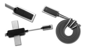
Micro-Measurements Sealed Weldable Strain Gages are specially designed for spot welding to structures and components. They are ideally used for applications where test or environmental conditions preclude clamping and curing an adhesively bonded gage installation. These gages
